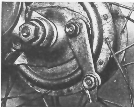
3.2 Release front brake cable and wheel nuts
