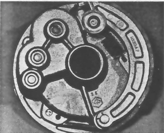
12.1a Rear brake has single brake shoe
