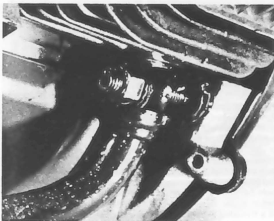
4.2a Exhaust system is retained by clamp ...
