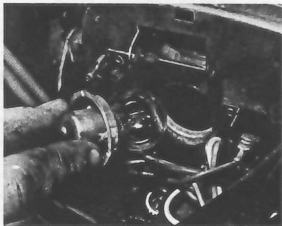
Displace contact to release headlamp bulb
