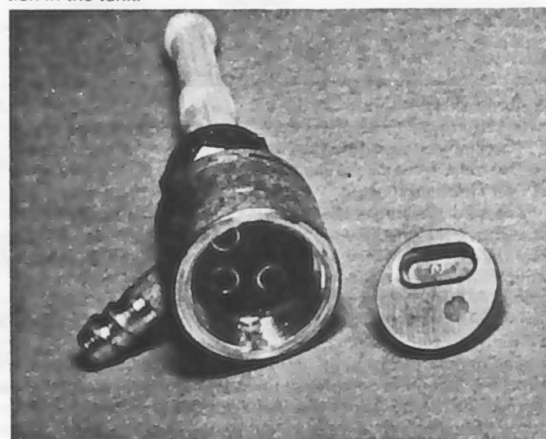
4.2b Petrol is channelled through slot in aluminium block
