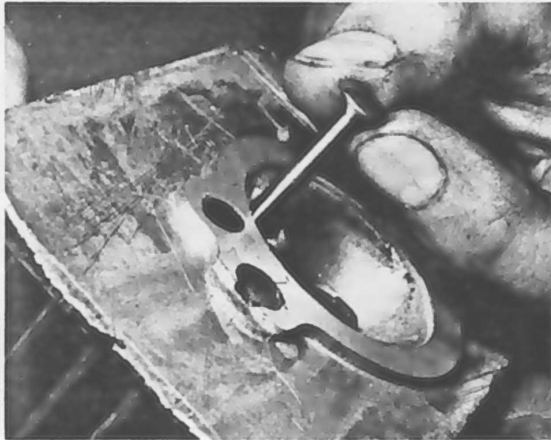
13.6c Valve can be removed from cylinder head
