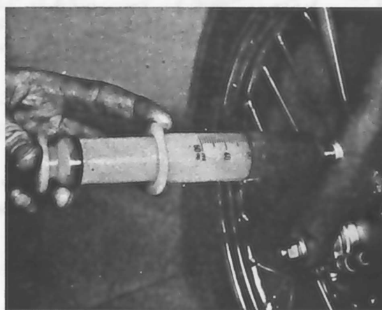
7.3d Refill fork legs to level hole
