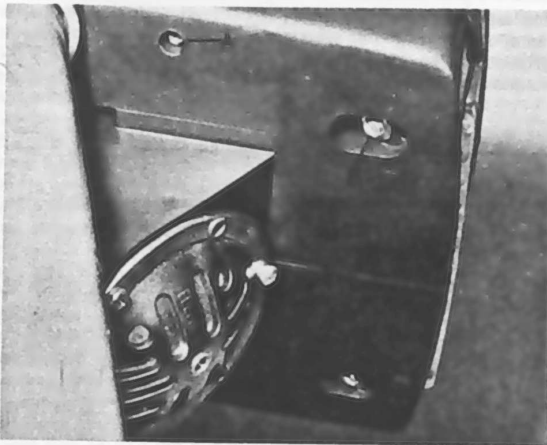
3.1a Note securing screws (A) and adjusting screws (B)
