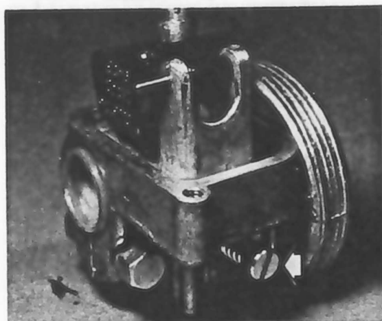
7.5a Refit float and pivot pin. Note throttle stop screw (arrowed)
