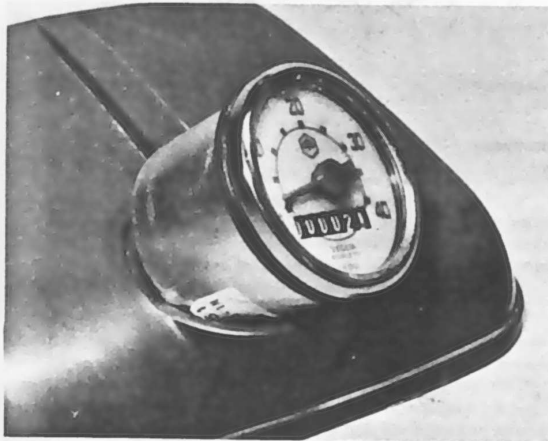
13.1a Speedometer is mounted in headlamp shell ...
