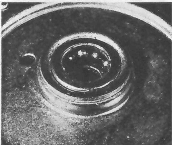
5.3 Balls are retained by steel ring
