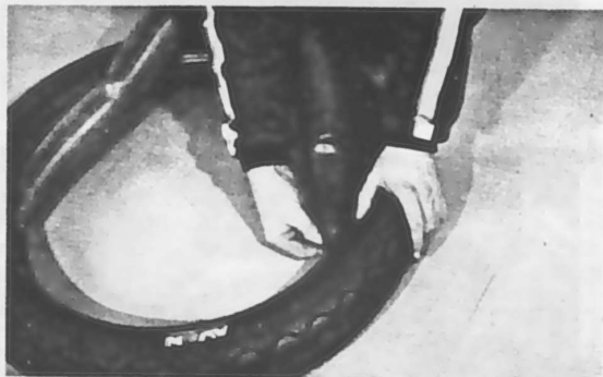
Tyre fitting: Inflate inner tube and insert in tyre
