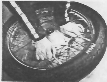
Use two levers to work bead over the edge of rim
